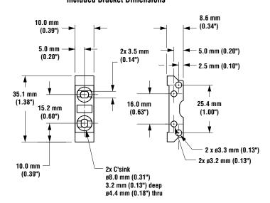
M3 Hardware included: Lock Washer (2) Flat Washer (2) Screws (2) Hex Nuts (2)
